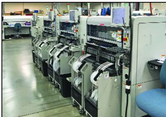
One of TSI's four new Yamaha SMT lines.
