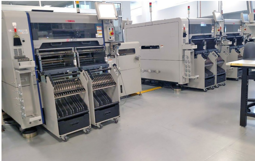
Three (3) YAMAHA Z:LEX YSM20 high-efficiency modular surface mounters in-line at World electronics. Their performance has been continuously supported by the team at Trans-Tec America, the leading distributor of Yamaha SMT equipment solutions in North America.
