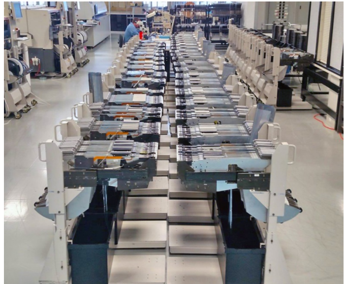
Feeders lined up and ready to handle the full high-mix range of SMT builds at World electronics.
