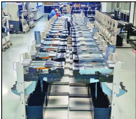
Feeders lined up to handle the full high-mix range of SMT builds at WORLD electronics.
