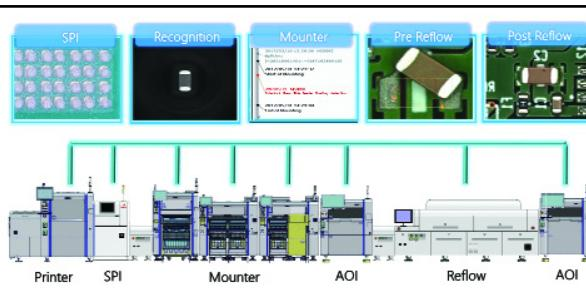
**SMT line with closed-loop feedback of SPI data to printer, AOI data to the mounter and the correlation of all data with traceability software.**
