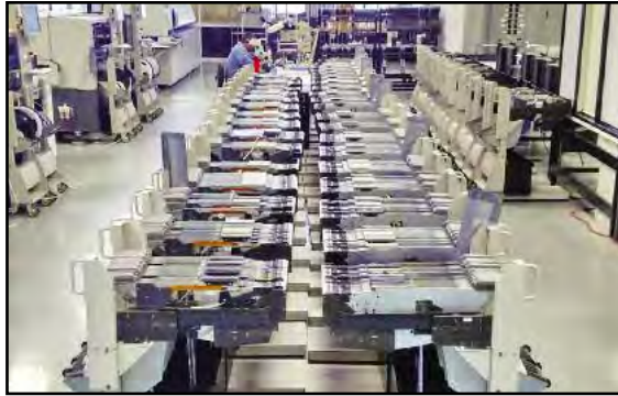
Feeders lined up to handle the full high-mix range of SMT builds at WORLD electronics.
