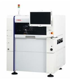
In addition to standard 2D AOI functionality, the YSi-V Series machines can be configured for high speed 3D inspection as well. Furthermore, the YSi-V has 4D capability by employing 4 additional off-axis cameras along with its main downward looking camera. With 4D capability, components can be inspected at 5 different angles, increasing object visibility around nearby components. Moreover, all five images can be later recalled at a repair station for better defect analysis.
